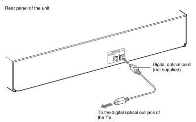
With a digital audio connection, the system receives a Dolby Digital multiplex broadcast signal and you can enjoy multiplex broadcast sound.
